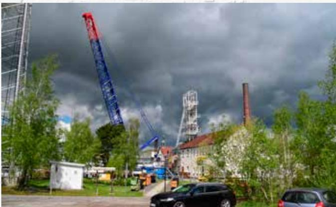
Liebherr LG 1750, Traglast: 750 t, 8 Achsen, Kranmotor: 455 kW
