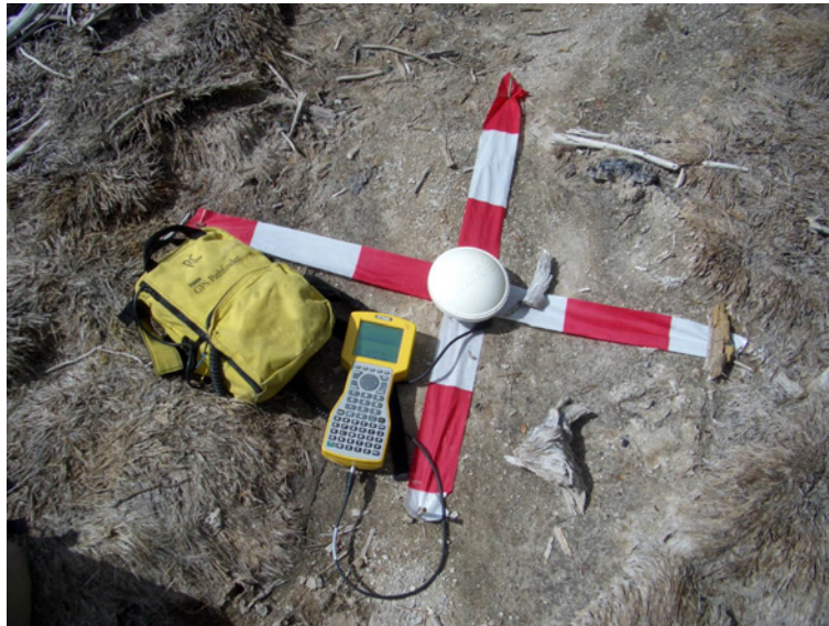
Figure 12: Differential GPS measurement of ground control point's coordinates
