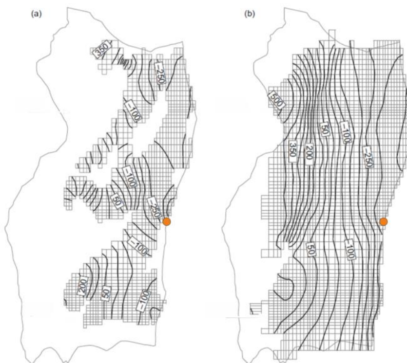
Figure 18: Water table elevations for (a) Upper Judea Group and (b) Lower Judea Group (Ben-Itzhak and Gvirtzman 2005). The study area is denoted
