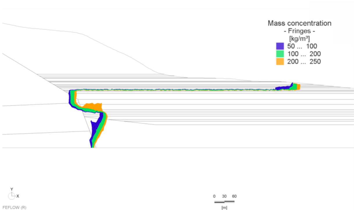
Figure 46: Mass concentration pattern (hydraulic aperture vs. depth, x:z = 1:1)
