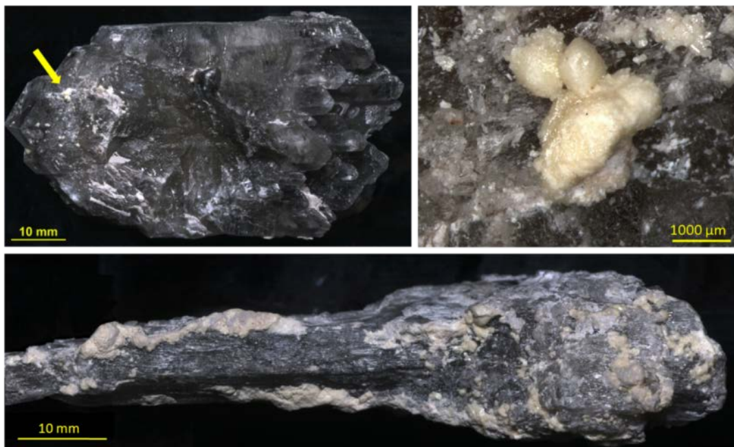
Figure 23: Large gypsum crystals with sulphur blooms on their surface. (Bottom) Gypsum crystal DC-SG-13c. (Upper Left) Gypsum crystal DC-SG-13d with the corresponding sulphur bloom DC-ES-13d (Right)
