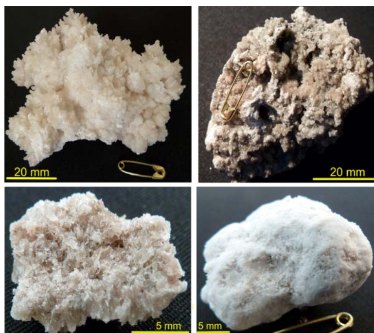
Figure 22: Variations of gypsum in the cave. (Upper left) DC-SG-15 was collected from the entrance of the cave. The mineral has distinct and stable crystals. (Upper right) DC-SG-14a was collected from the outermost gypsum layer at the narrow passage to the crystal chamber. The mineral has a rough and firm surface, composed of gypsum needles. (Lower left) DC-SG-9c was collected from the crystal chamber. Like the samples depicted in the upper photos, it presents the outermost gypsum layer of the sampling site. In contrast to the others, it is a relatively loose, brittle accumulation of small, young gypsum needles. (Lower right) Sample DC-SG-9b, a soft, homogeneous, and chalky gypsum from the layer underneath DC-SG-9c.
