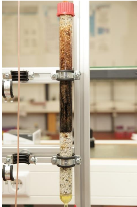
Figure 23: Photograph of the multi system at the end of the defluoridation experiment (70 days).
