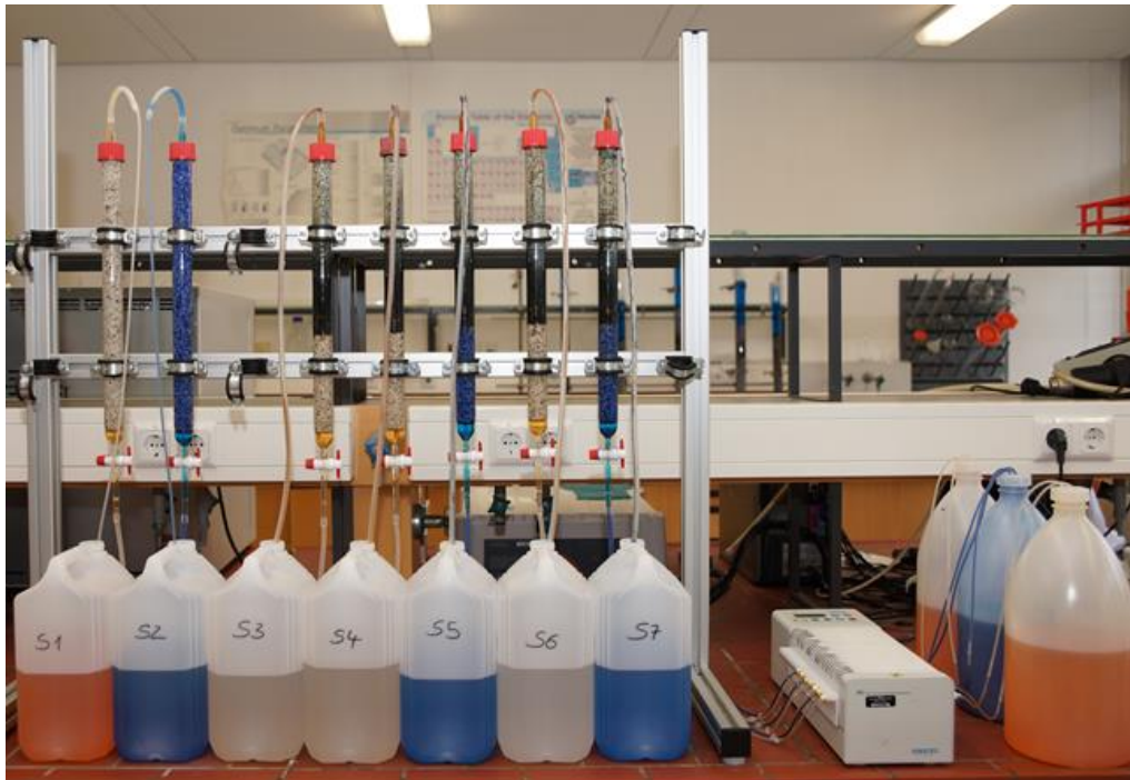
Figure 26: Photograph of the columns from experiment 1 after 21 days of dye “flushing”.
