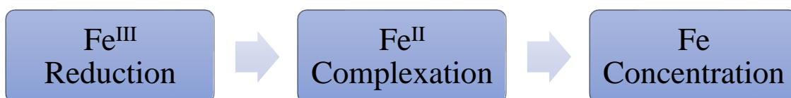
Figure 9: Preparation process of samples for the dissolved iron measurement (modified after Phukan 2015).
